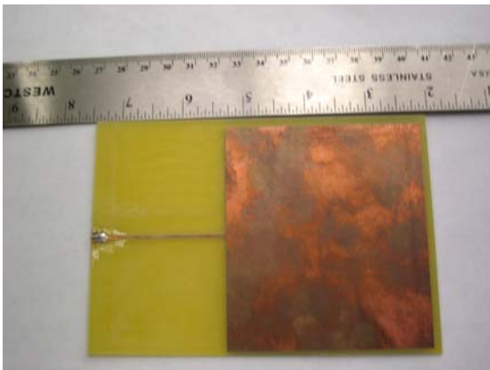
Figure 4.4: (a) Layout of monopole antenna with capacitive patch; (b) Final antenna after milling
